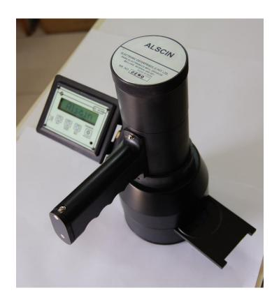
**α-Scin** uses micro controller for counting, menu display and key board functions. Pulse processing electronics generates the TTL shaped pulses fed as input to the counter. Typical Alpha Counting efficiency is better than 22%.
