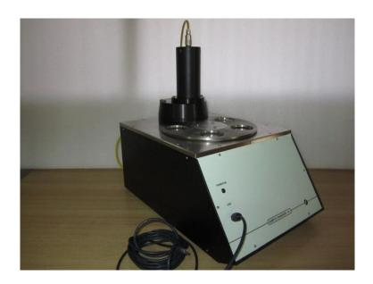
Para Model ASC-05A / ASC-10A Automated Sample Changer - Alpha Counter is a versatile indigenously developed system for Alpha radiation counting of samples on 25 mm (1") or 51 mm (2") diameter filter papers or planchets.
