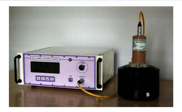
Dual Channel Alpha Beta Counter model **PNC-\alpha\beta** is a micro-controller based, economical, stand alone, mains operated instrument for Dual Channel Nuclear Counting application for Alpha – Beta radiations. It is a versatile instrument designed to cater the counting application requirements.
