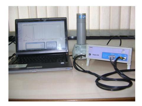
GSpec SA is a 1K Multichannel Analyzer with HV Supply and Spectroscopy Amplifier. It is a mains operated instrument for NaI(TI) detector based spectroscopy.
