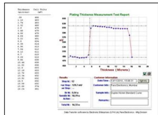
Instrument determines the points (thresholds) at which change in layer takes place. Due to non-uniform coating, sometimes the instrument may show wrong results. In such cases, transfer the data to PC and run the software. In the software, user can change the thresholds by looking at the graph displayed on screen. This helps to get the proper and more accurate results.
