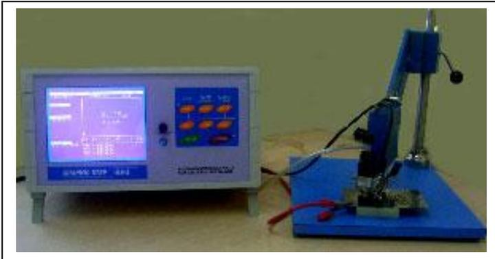
Graphic Step is an advanced version of our earlier Smart Step. It works on Coulometric Principle. It measures plating thickness of various metallic coatings on variety of base materials. Step measurement of Duplex and Triplex Nickel is also possible in this instrument.
