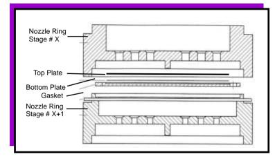
A typical stage is shown alongside. Nozzle rings are made of aluminium alloy of grade 6061, collection and impaction plates are of stainless steel, connecting adapters and fasteners are of brass. The unit is made leakproof with the use of neoprene gaskets
