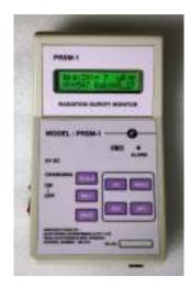
Portable Radiation Survey Monitor Model PRSM-1 is a micro-controller based, portable battery operated instrument for measurement of environmental/ field dose rate of Gamma and X-ray radiations. It is useful for Health Physics applications in Radioisotope Laboratories, Nuclear Power Plants and nuclear medical centres.
