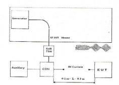
Noise in the above frequency range was superimposed on AC mains using a 150  $\Omega$  CDN and the operation of the equipment was monitored.
